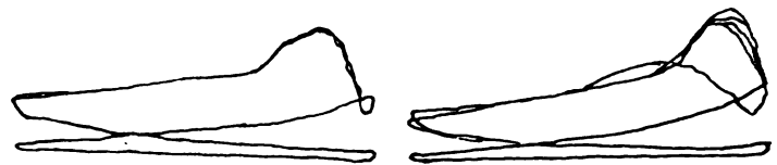
Fig. 22 (left)—Actual diagram of late firing Fig. 27 (right)—Very poor mixture and late exhaust
